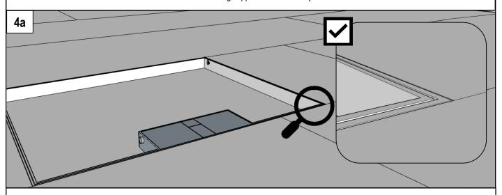
The trim edge of your floor box lid and lid frame should be flush with final floor...
