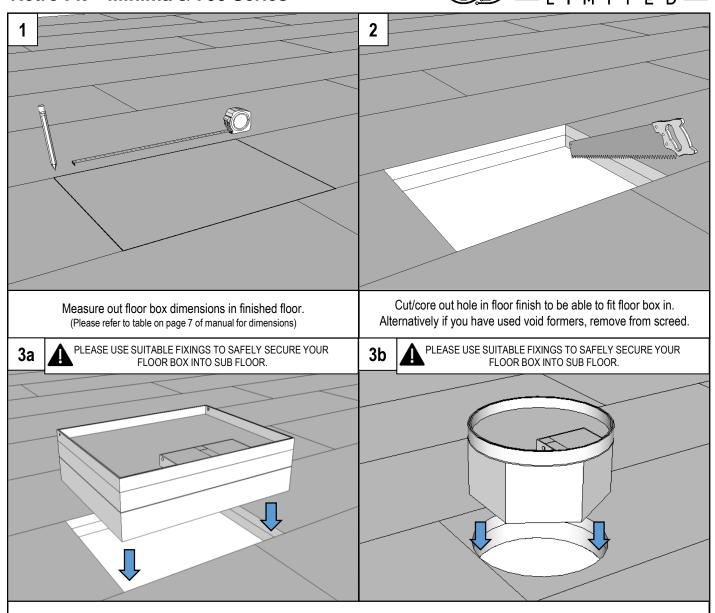
Lower & fit floor box into hole. You will need to consider how the floor box is fixed and supported in floor. Support batons or plinths may be needed in the sub floor as load bearing support aides. Securely fix floor box into sub floor.
